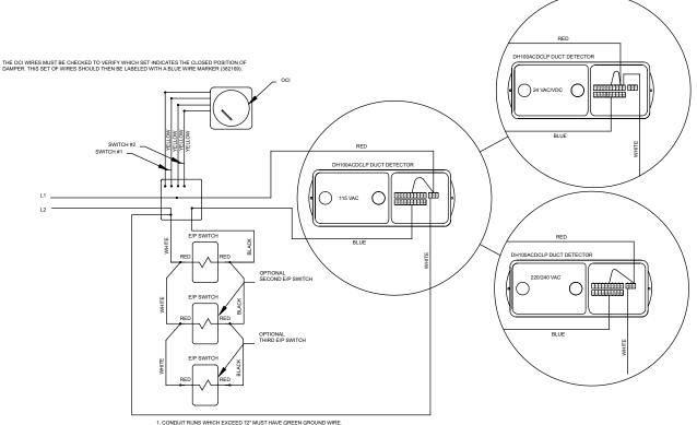
1. CONDUIT RUNS WHICH EXCEED 72" MUST HAVE GREEN GROUND WIRE. 2. FLEX CONDUIT MUST BE SECURED WITH A CONDUIT CLAMP (45226) WITHIN 12" OF CONDUIT TERMINATION AT THE HANDI-BOX OR ACTUATOR. CONDUIT RUNS MUST ALSO BE SECURED ALONG SLEEVE AT A MAXIMUM OF 24" ON CENTER.
